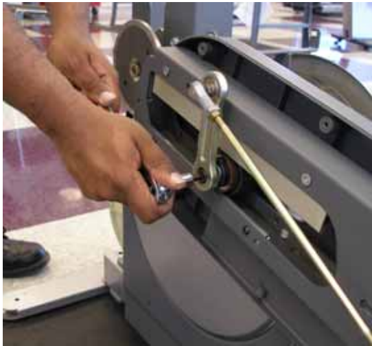
Fig. 5: removing the crank extension bolt
